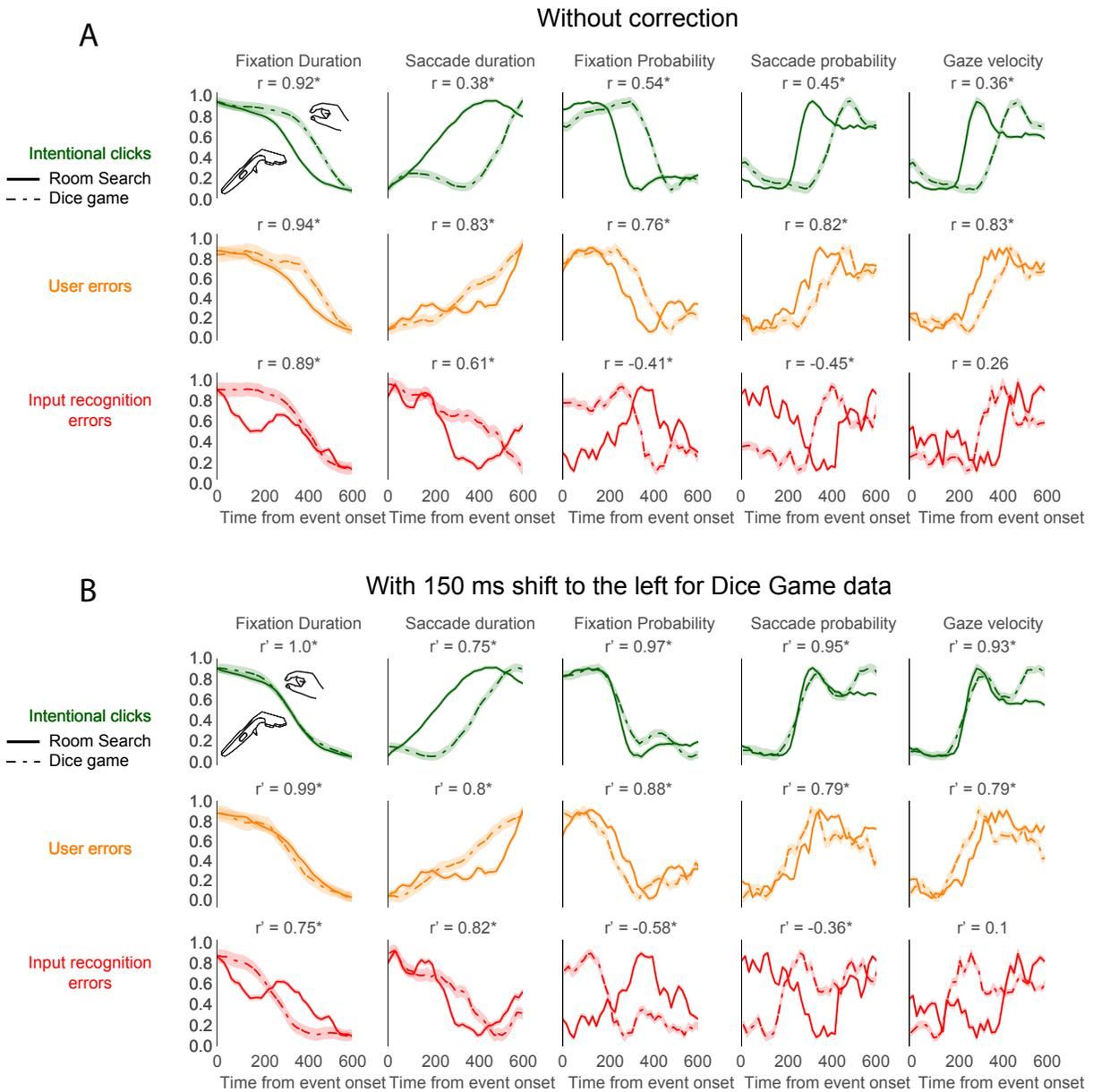
**Figure A3: Gaze features for different input event types for the Room Search task with the controller key press (solid line) and the Dice Game task with the gestural input system (broken line) without any temporal shift (A) and with 150 milliseconds temporal shift to the left (B). This figure uses the same format as Fig. 9.**
